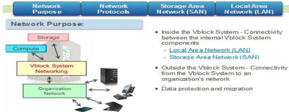
Vblock System servers have no storage and their OS files are stored on storage devices. Instead of separate IP and SAN switches, Vblock systems can be built with Cisco Unified Switch. A unified switch can perform tasks associated with both IP and Fibre Channel networks. However, a separate LAN and SAN switch would have more ports than a Unified switch. Hence, we have two options to consider for Network in VBlock Systems:
