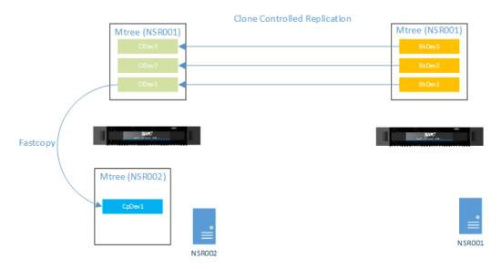
The diagram above shows the basic premise. A NetWorker server (NSR001) has backups in the production data center and clones in the DR data center. The clone devices can be fast copied to the mtree owned by the DR NetWorker server (NSR002). NSR002 can now scan the fast copied device and make use of the data on this device. If we have separation of index and backup data then we need to fast copy both the data clone and the index clone device.
