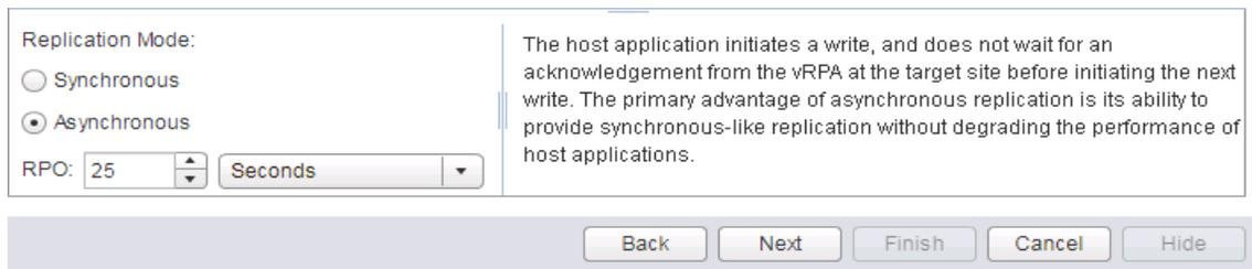
**Figure 15 – The PRO and Replicate Mode settings in protection wizard**
