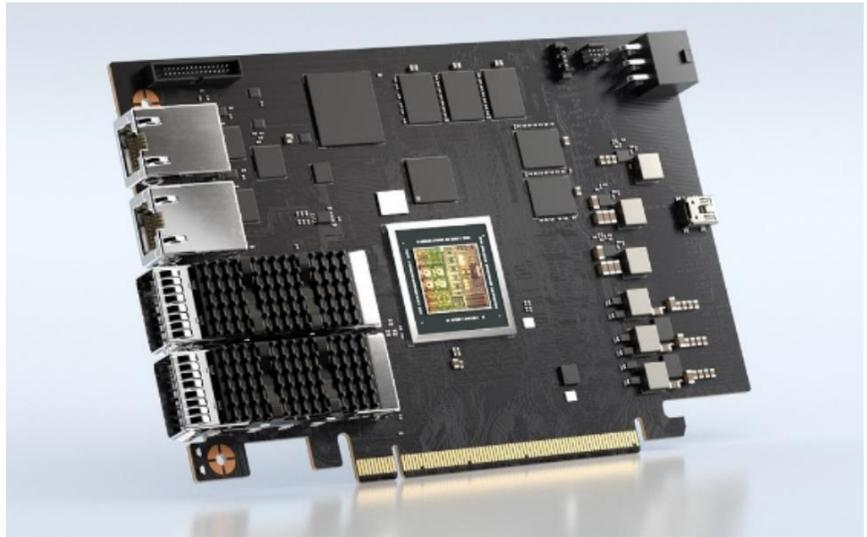
**Figure 1: NVIDIA BlueField-2 SFF form factor, an example of a DPU [Ref 4]**
