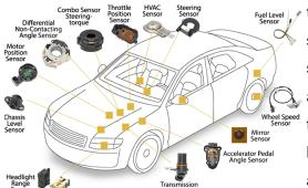
that triggers the process to run the engine. Relevant sensors such as this coolant temperature sensor store digital values in specific addresses in volatile ECU memory. The illustration to the left shows a modern car can have dozens to hundreds of sensors that monitor important functions and generate tens of thousands of status messages.<sup>3</sup>
