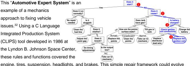
engine, tires, suspension, headlights, and brakes. This simple repair framework could evolve into a more detailed and model-specific mechanics expert system to help diagnose issues based on customer answers and OBD-II data points, helping to quickly correct an issue.
