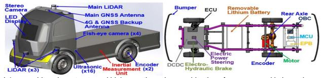
L4 was achieved on streets and highways through a combination of cameras, multi-channel LiDAR, ultrasonic short-range sensors, and RADAR.<sup>84</sup> The cargo bay is not shown, but you can see the Inertial Measurement Unit, electric motors, removable lithium-ion battery, ECU, Motor Control Unit (MCU), Electric Power Steering, Electro-Hydraulic Brake, Electronic Parking Brake (EPB), On-board Battery Charger (OBC), and Direct-Current-to-Direct-Current (DC/DC) converter.
