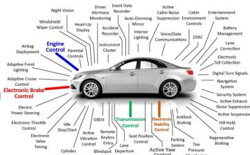
**Electronic Stability Control** (**ESC**) improves stability algorithmically by detecting and reducing traction loss through speed sensors on each wheel, steering wheel position, and actual vehicle path by sending control sequences to individual brakes through the **EBCM**. An ECU generally runs a single application and is responsible for the algorithmic processing of sensor inputs.
