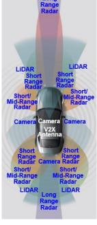
LiDAR can use various non-visible infrared light wavelengths between 850 – 1550 nm, each with advantages and disadvantages. A green visible 532 nm laser is not used since it would wavelength Comparison distract other drivers. Infrared 905 nm lasers could hurt the retina if the range exceeds 100 meters. Frequencies of 1550 nm are safer
