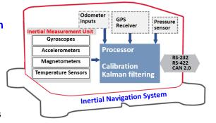
a linear quadratic estimation of sensor data over time to remove noise inaccuracies. 132
