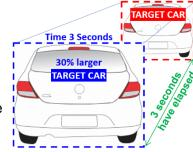
display a collision alert and sound warning chimes.<sup>49</sup> It might close the windows, adjust seat position and belts, and take other actions to help reduce injury. Whereas an average driver needs 1.4 seconds to apply a vehicle's brakes in an emergency, the ADAS needs less than 0.1 seconds. That 1.3-second improvement can save 180 feet of stopping distance at 56 MPH.<sup>50</sup>
