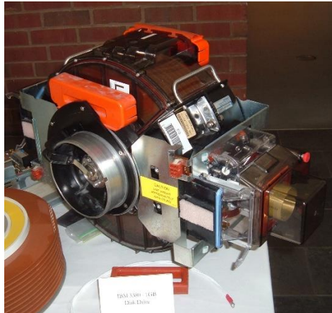
Figure 2: 1980s IBM 3380 disk drive (source: Wikipedia 2 )
